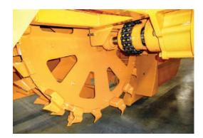
A trencher wheel mounts next to the platform, the pot-setting machine excavates a ditch deeper and wider than the pot to be set, lays down the drain tile in the bottom of the ditch and an irrigation hose along the side of the ditch. Workers ride on the platform and place pots in the ditch at regular intervals. Metal lids are placed over the pots to keep dirt out until the planted pots are inserted.
